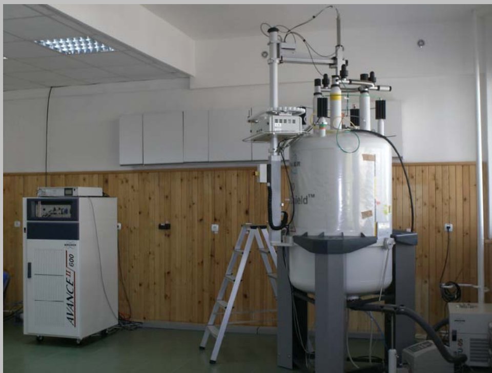
NMR spectrometer Bruker Avance II + 600 MHz
