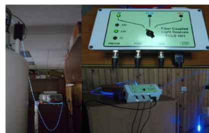
LED control unit and optical fiber to the NMR tube used for “ in situ ” UV-irradiation NMR spectroscopy
